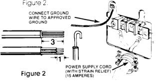
4. Connect a separate copper grounding wire (No. 10 minimum) to a grounded cold water pipe<sup>+</sup> by means of a clamp and then to the frame of the appliance at the external grounding connector. Use Part No. 685463 grounding wire and clamp assembly. Do not ground to a gas supply pipe. Do not connect should **not** be used.
